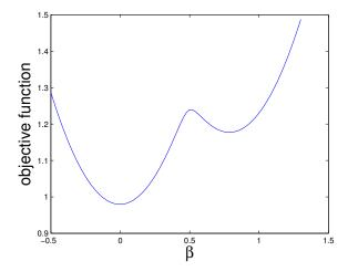
Figure 2: Example for multiple local minima in the least squares objective function  $L(\beta)$ . The global minimum can be found close to the true value  $\beta^0 = 0$ , but another local minimum exists around  $\beta \approx 0.8$ , which renders the FOC inappropriate for defining the estimator  $\hat{\beta}$ .
